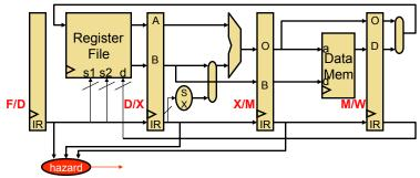
• Compare F/D insn input register names with output register names of older insns in pipeline
