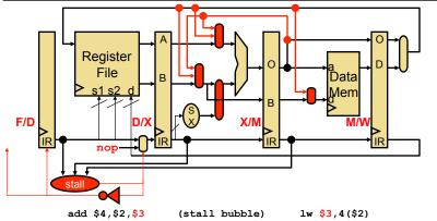
Stall = (D/X.IR.Operation == LOAD) && ((F/D.IR.RegSrc1 == D/X.IR.RegDest) || ((F/D.IR.RegSrc2 == D/X.IR.RegDest) && (F/D.IR.Op != STORE))
