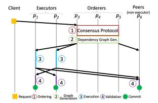
Fig. 3. The Flow of Transactions in ParBlockchain
