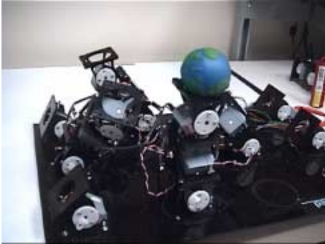
Figure 6: Four arms with three degrees of freedom each, demonstrate passing a small ball from arm to arm.
