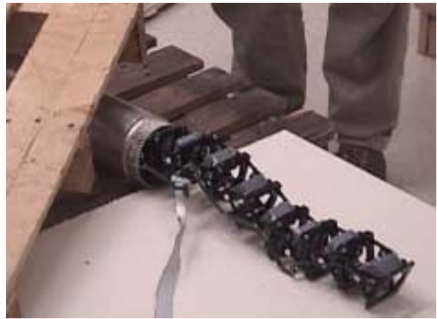
Figure 7: Sinusoid gait moving through rubble (10 cm pipe)
