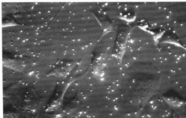
Figure 3. Bovine aortic endothelial cells seeded in the cell culture chamber. On the surface of each cell are polystyrene microspheres (white dots). Cell deformation can be determined by measuring the change in distance between these microspheres under hydrostatic loads.
