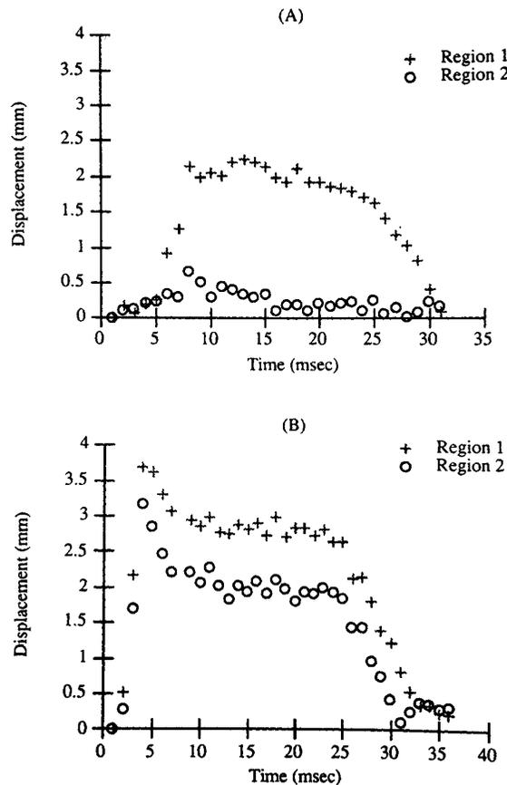
**FIG. 5.** Peak displacement ( $\delta$ ) of surrogate brain tissue caused by cortical impact for (A) unilateral and (B) bilateral craniotomy configurations. Using a contralateral craniotomy moves surrogate tissue across the sagittal midline and reduces the movement of surrogate material through the foramen magnum.
