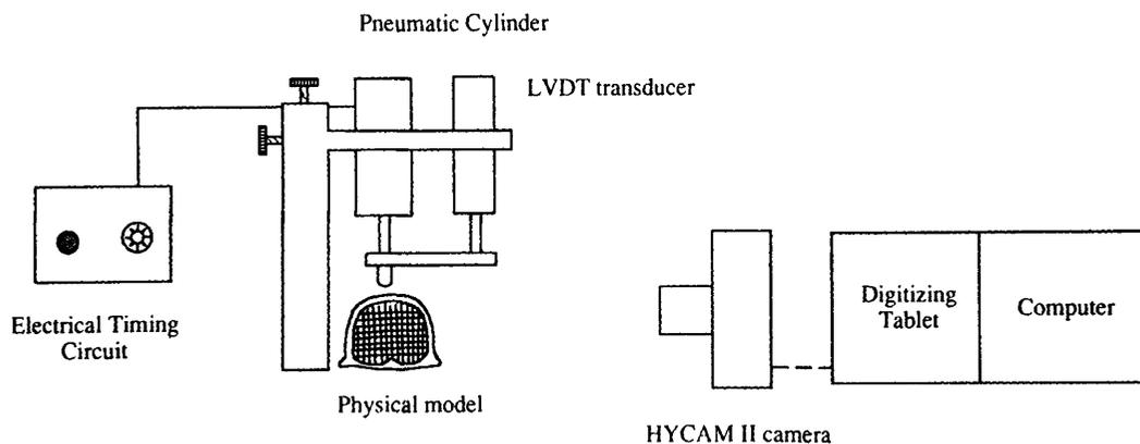
**FIG. 1.** Schematic of cortical impact apparatus, consisting of a pneumatic cylinder coupled to two independently controlled solenoid valves. Pressure supplied to the solenoid valves permitted varying the impact velocity, and a timing circuit controlling the solenoid valve operation allowed the indentation duration to vary across a wide range (25 msec–3 sec).
