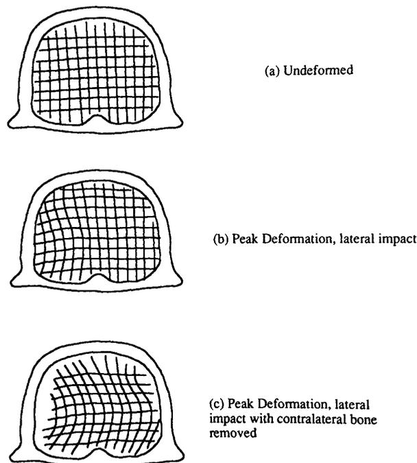
**FIG. 4.** Digitized reconstructed images of coronal plane grid deformation caused by lateral impact for (b) unilateral and (c) bilateral craniotomy configurations. Note the pronounced displacement of the grid pattern across the sagittal midplane when a contralateral opening is used (c).
