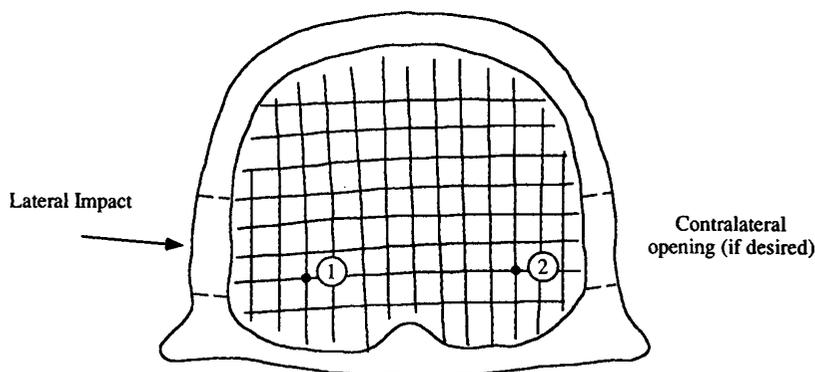
**FIG. 3.** Schematic of areas examined in the physical model tests, intended to encompass regions both near (1) and remote (2) from the impact site.
