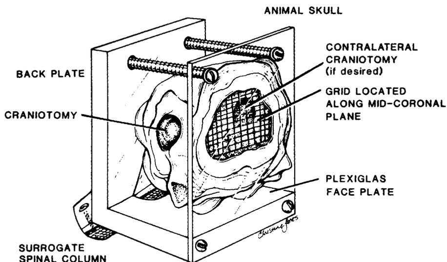
**FIG. 2.** Illustration of physical model used to investigate cortical impact. A cat skull was cut coronally, fitted with a surrogate cervical spinal column, and filled with a silicone gel material intended to simulate the mechanical properties of brain tissue. Distortion of a grid located in the midcoronal plane was used to measure the strain caused by lateral impact to the cortex.
