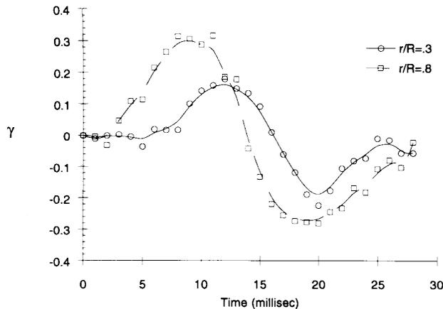
**FIG. 3.** Strains measured in the surrogate modeling tests patterned the biphasic acceleration, and were larger along the periphery ( $r/R = 0.8$ ) of the model when compared to the inner core ( $r/R = 0.3$ ).
