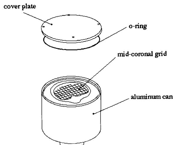
**FIG. 1.** Illustration of the physical model used in this study. A clean, dried porcine skull was embedded within an aluminum can and filled with a silicone gel that acted as a surrogate for brain tissue. An orthogonal grid placed between two gel layers was used to estimate the mechanical response of the brain surrogate to a coronal plane, rotational acceleration.
