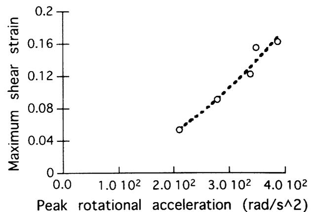
**FIG. 4.** Several physical model tests were conducted to characterize the response of a region approximating the subcortical white matter to changes in the peak rotational acceleration and peak change in rotational velocity. A critical strain value for axonal injury (0.1) yielded estimates for the loading conditions required for mild DAI.
