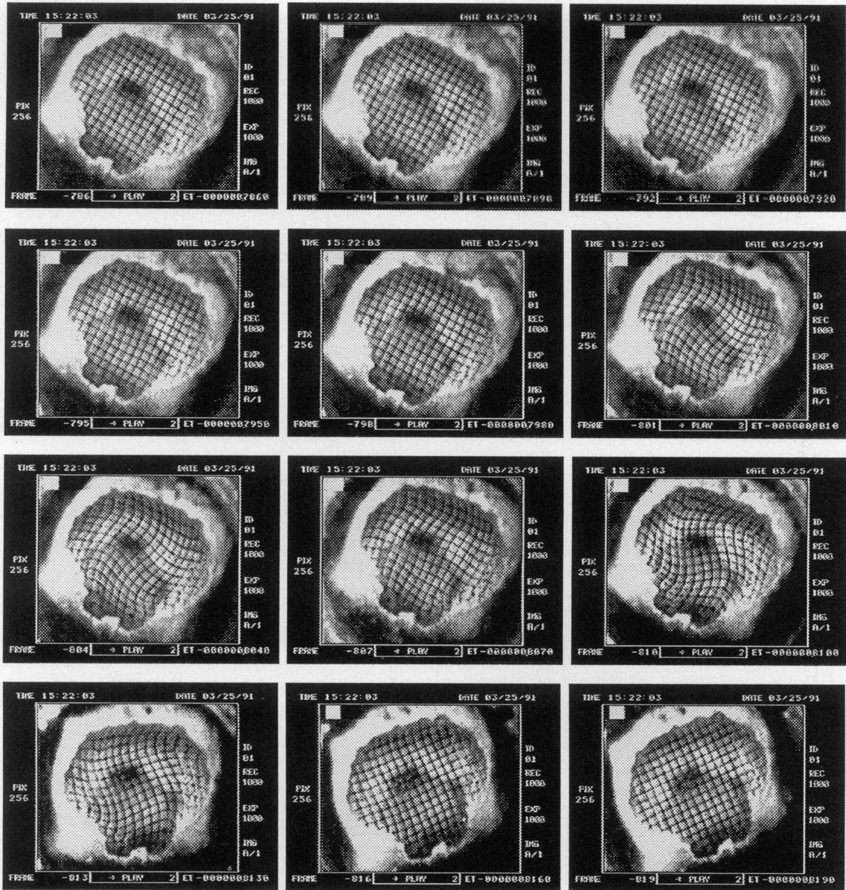
**FIG. 2.** High-speed video (1000 frames/s) captured the distortion of the grid within the physical model in response to a biphase rotational acceleration/deceleration. Analysis of a consecutive series of grid frames allowed for the calculation of strain throughout the grid plane of the physical model.
