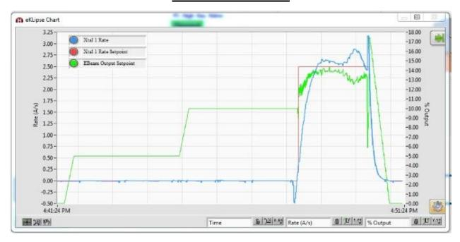
Thickness deposited: 20 nm Rate: 2.5 A/sec
