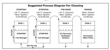
For detailed cleaning procedures, refer to the section describing the 562-S Stripper.
