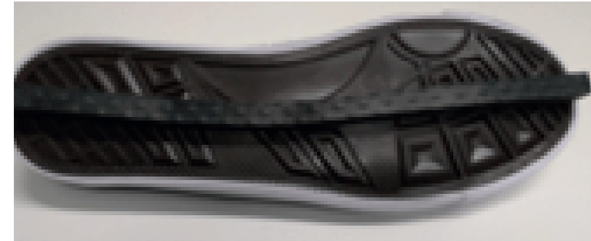
Figure 1. LesSchuh, a shoe on which using the mediolateral ankle strategy is impossible. This is achieved by a flexible ridge along the sole, which makes the shoe resemble a skate. The flexible ridge allows for normal push off.
