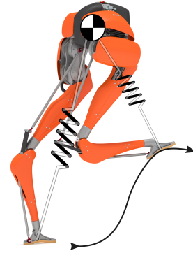
Fig. 1: The policy learns to choose actions in Cassie’s task space in terms of foot positions, which essentially preserves the robust action space based on reduced-order models. Along with the analytical controller that maps actions into joint torques, the proposed learning approach facilitates natural action representations for what the bipedal locomotion policy should learn in the most meaningful way.
