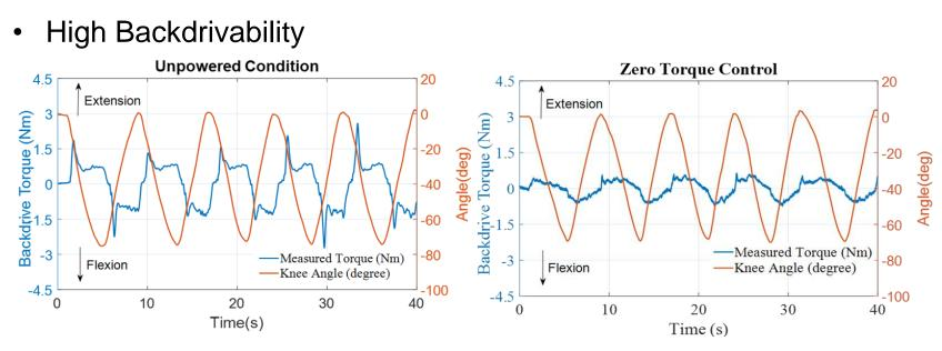
The backdrivability performance of the knee exoskeleton in the unpowered mode and zero torque tracking control. The average backdrive torque is 0.92 Nm and 0.34 Nm respectively
