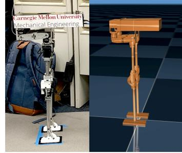
Fig. 1: Left: Real life prototype of the flamingo robot. Right: Robot model simulated in MuJoCo simulation environment.
