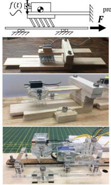
Once this first prototype proved that the concept would work a second prototype linear actuator was fabricated from laser cut acrylic and plywood materials to more carefully experimentally
