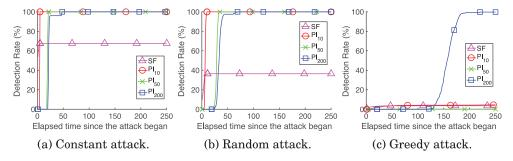
Fig. 7. Time to detection plots under the three classes of attacks on the simulated systems.
