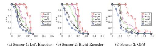
Fig. 4. Empirical plots of the proportion of faults in a window (e/w) against the error bound  $(\epsilon)$ .
