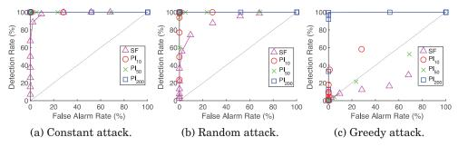
Fig. 8. Detection Rate vs. False Alarm Rate under the three classes of attacks on the simulated systems. Dotted black lines denote  $45^{\circ}$  lines. Solid lines connect points for a clearer presentation.
