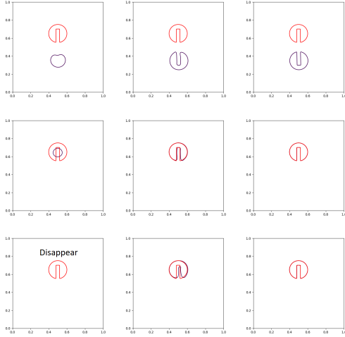
Fig. 10. 2D Zalesak's disk. Results shown are Semi-Lagrangian (left), BFECC (middle) and BiMocq 2 (right) at t = 79 seconds (top), t = 628 seconds (middle) and t = 1884 seconds (bottom). Note that our method can almost perfectly match the original shape after three revolutions.
