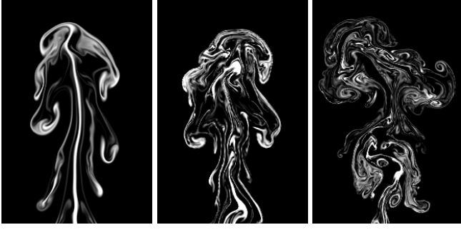
Fig. 3. 2D simulation of a released smoke in a tank, from left to right: results obtained with Semi-Lagrangian simulation, results from only advecting the density field with BiMocq 2 , and results obtained by applying BiMocq 2 to both velocity and density fields. Note that simply improving the accuracy of density advection is able to bring more detailed flow field as the density field affects the flow simulation via buoyancy force. With BiMocq 2 used for both fields, the flow becomes more energetic due to better momentum conservation.
